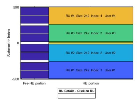
Similarly, for a 160 MHz transmission, the central 26-tone RU in each 80 MHz segment can be optionally used. Each central 26-tone RU can be enabled using name-value pairs when creating the wlanHEMUConfig object. In this example only the upper central 26-tone RU is created. Four 242-tone RUs, each with one user are specified with the allocation index [200 114 114 200 200 114 114 200].
