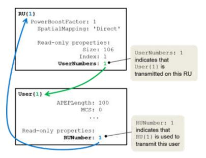
This allows the properties of an RU associated with a User to be accessed easily:
