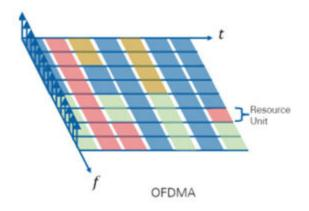
The values specified by AllocationIndex correspond to the 8-bit indices in the first column of IEEE P802.11ax/D2.0 [1], Table 28-24 (RU Allocation subfield). These 8-bit RU Allocation subfield values indicate the RU assignment and the number of users per RU. Together the RU assignment and the number of user fields per RU indicate the number of user fields in the user-specific field of HE-SIG-B.
