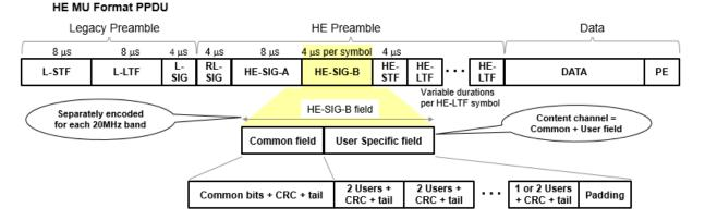
When SIGB compression is not used, the HE-SIG-B field includes the Common field. The Common field carries the RU Allocation subfields in one or two content channels. Depending on the PPDU bandwidth, the Common field can contain multiple RU Allocation subfields. Frequency domain mapping of channel content into the Common field is discussed in Section 28.3.10.8.3 of [1].
