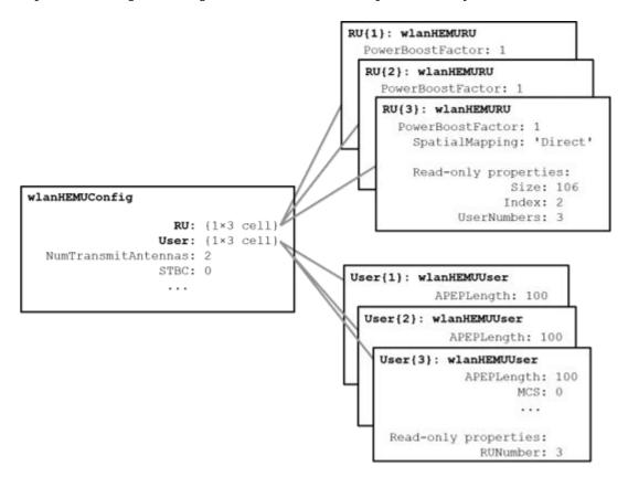
In this example, three RUs are specified by the allocation index 128, therefore cfgMU.RU is a cell array with three elements. The index and size of each RU are configured
