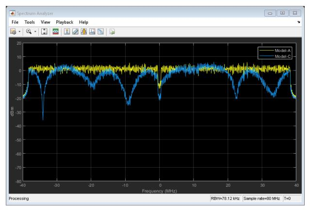
As expected, the frequency response of the model-A signal is flat across the 80 MHz bandwidth. Conversely, the model-C frequency response varies because its coherence bandwidth is much smaller than the channel bandwidth.
