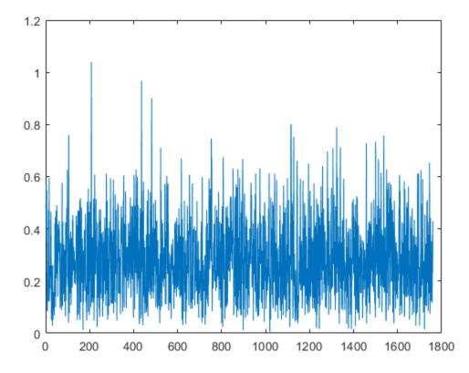
Extract the L-LTF from the received PPDU using the start and stop indices determined by the wlanFieldIndices function. Demodulate the L-LTF and estimate the channel coefficients.
