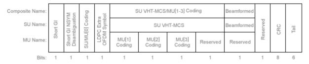
The VHT-SIG-A field includes these components. The bit field structures for VHT-SIG-A1 and VHT-SIG-A2 vary for single user or multiuser transmissions.
