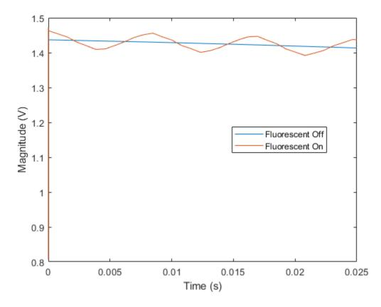
Fluorescent lighting introduces a Doppler component at twice the power line frequency (120 Hz in the U.S.).
